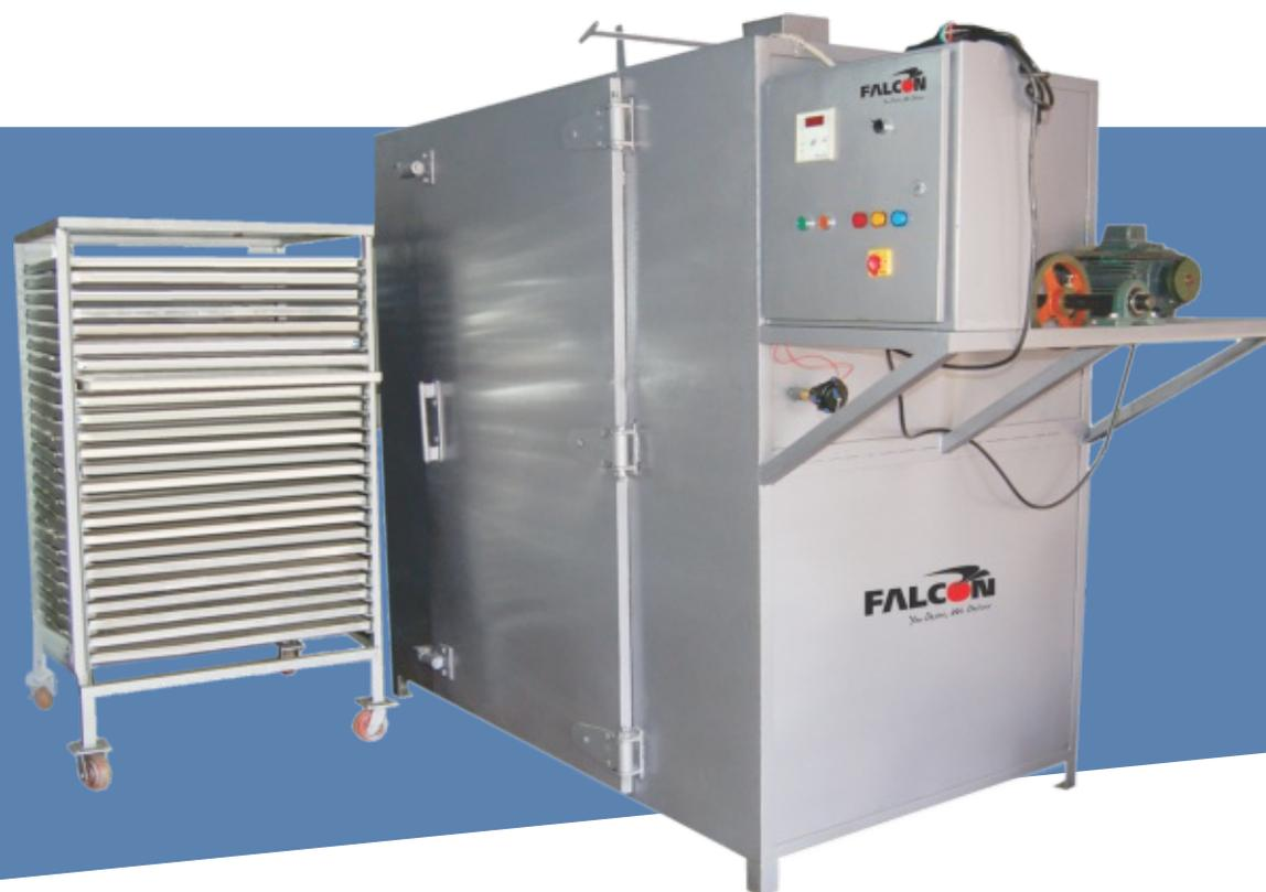
Designed for uniform circulation of hot air in the drying chamber. Electrical / Steam.
