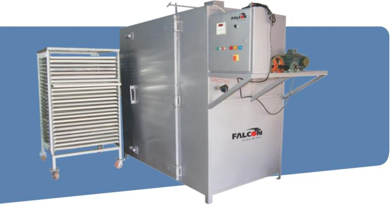
Designed for uniform circulation of hot air in the drying chamber. Electrical / Steam.
